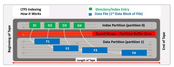
paste files to tape in the same familiar way as performed on disk, SSD, CDs, or DVDs via the LTFS GUI.
