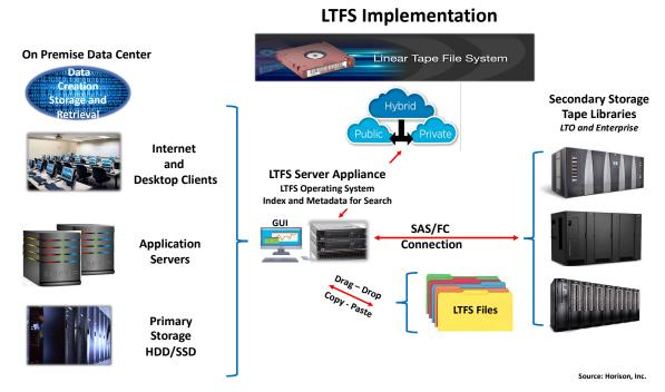
Key point: With LTFS, tape still requires sequential access to data but acts more like disk. LTFS is <u>not a</u> <u>disk replacement</u>, but it improves time to first byte compared to any previous tape format.
