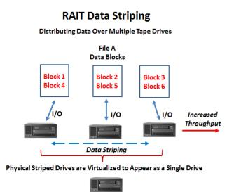
data within a stripe. The stripe capacity is limited to the capacity of the lowest capacity drive in the array. The minimum size of a RAIT stripe is 3 and can range to 16 drives depending on the software used.
